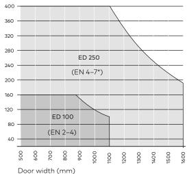
The operators ED 100 and ED 250 are suitable for most swing doors provided that the combination of door width and door weight lies within the defined functional area.
